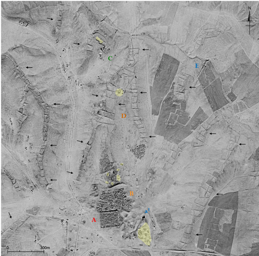
114 Figure 4 - Umm ar-Rasas. Hexagon KH9 images 1974/12/01, ground resolution: 1.20-0.60 m. Featured: A Roman 115 castrum; a¹ hydraulic reserve; B Byzantine and Umayyade settlement; C Stylite tower complex; D System of 116 irrigated plots (channels and dams); E the dam. Quarries and material extraction points are highlighted in 117 yellow, whilst arrows indicate hydraulic channelling systems (Hexagon acquired from USGS and edited by 118 Francesca Di Palma).
