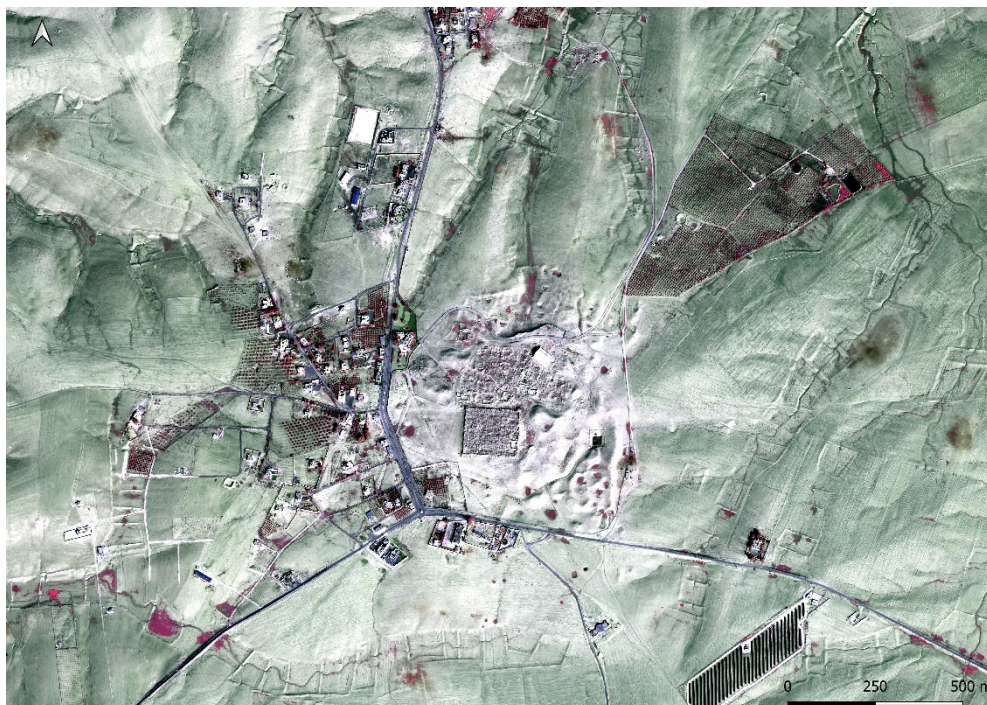
227 228 229 230 231 232 233 234 235 236 237 238 239 240 241 242 243 244 245 246 247 Figure 8 - Pansharpended product of the datafusion technique by panchromatic and multispectral data 248 of Pléiades Neo-04 image (processing and editing by Ilaria Miccoli).
