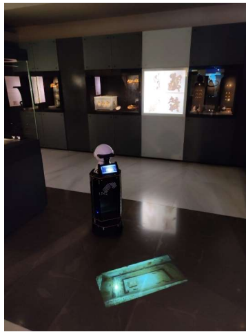
Figure 18 – The screen is also projected on the floor for better visualization of the information. c
