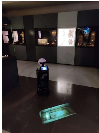
Figure 18 - The screen is also projected on the floor for better visualization of the information.
