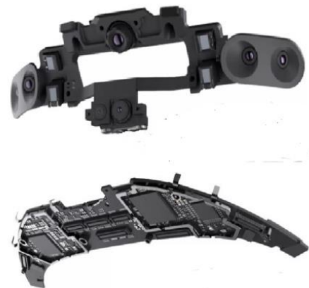
Figure 3 Sensors (upper) and processing units (lower) https://developer.microsoft.com/en-us/windows/mixed-reality/hololens_hardware_details
