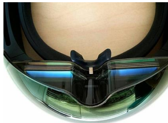
Figure 4 Optical units viewing bottom of HoloLens
