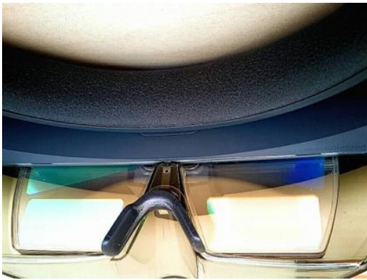
Figure 5 See-through holographic lenses (light waveguides)
