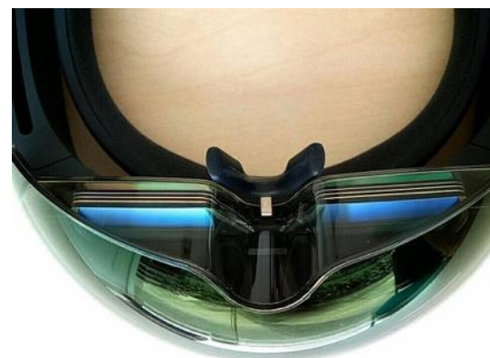
Figure 4 Optical units viewing bottom of HoloLens
