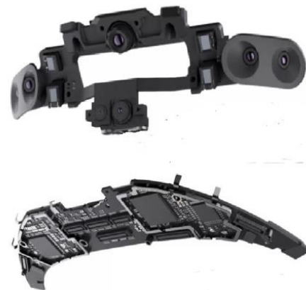
Figure 3 Sensors (upper) and processing units (lower)
