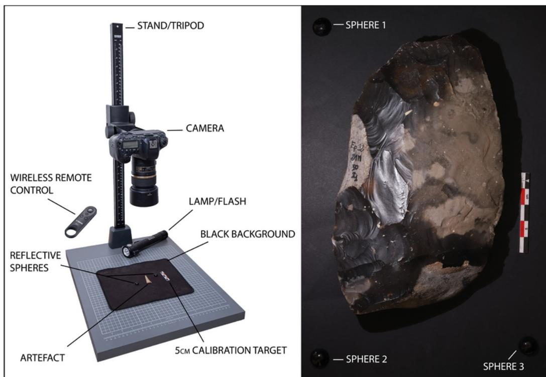
512 **Figure 8** - Left: installation and equipment required for RTI acquisition.
