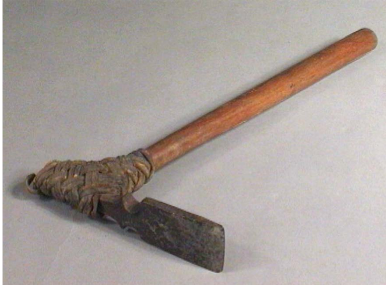
Fig 7. Adze from Minangkabau region, Indonesia. Wood handle, metal blade attached with split cane lashing. The handle is 40cm long and the iron blade is 14cm long. Wereldculturen Museums RV-268-372, accessioned in 1881. Creative Commons 4.0 International License.
